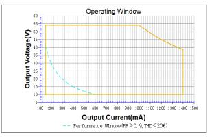
It's important to set the output current (AOC value) according to the LED voltage and make sure the power is within 54 W + 5%.
