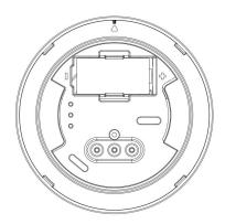
Key One: PIR Sensitivity Adjustment. The PIR sensitivity has four adjustable levels: 25%, 50%, 75%, and 100%. Short press the button to switch between levels. A green light blinking once indicates the 25% level, a steady green light indicates the 50% level, a green light blinking once followed by a second light blinking indicates the 75% level, and both lights steady indicate the 100% level.
